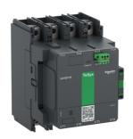
High power contactor, TeSys Giga, 4 pole (4NO), AC-1 <=440V 305A, standard version, 48...130V wide band AC/DC coil
